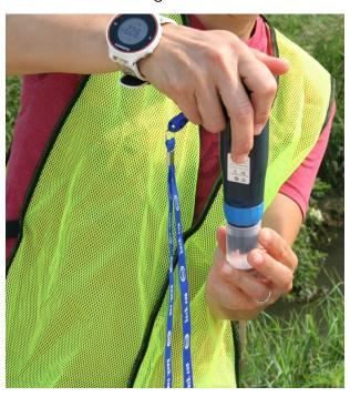
Finally, we received a grant from the Regional Development Authority, and with these funds were able to purchase a Hach Colorimeter. This meter provides much more accurate readings for orthophosphate levels than our previous method of in-field color comparators.
